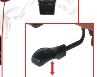
Press and hold down the seat slider paddle and move the seat to the desired location and release the paddle to lock the seat in place.
